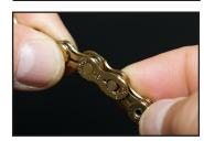
5. Press both halves of the MissingLink connector together
